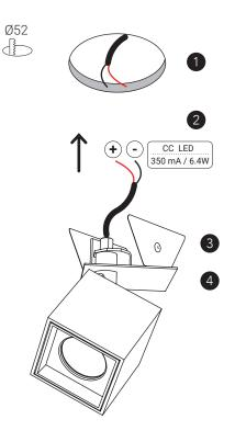
1 Make an opening of diameter 52mm in the ceiling.
