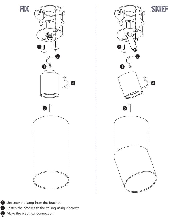
4 Screw the lamp back onto the bracket.
